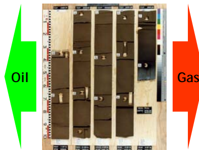
Fig. 5. Middle Jurassic oil stained reservoir sandstones of the Sto Formation from well 7121/5-1.
